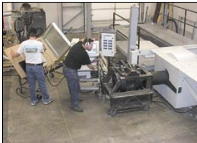
SuperFlow technicians measure inertia, aerodynamic and friction losses on AWD AutoDyn.
